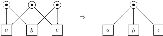
Fig. 7. A distributable net which is not considered distributable in [9], and its implementation
